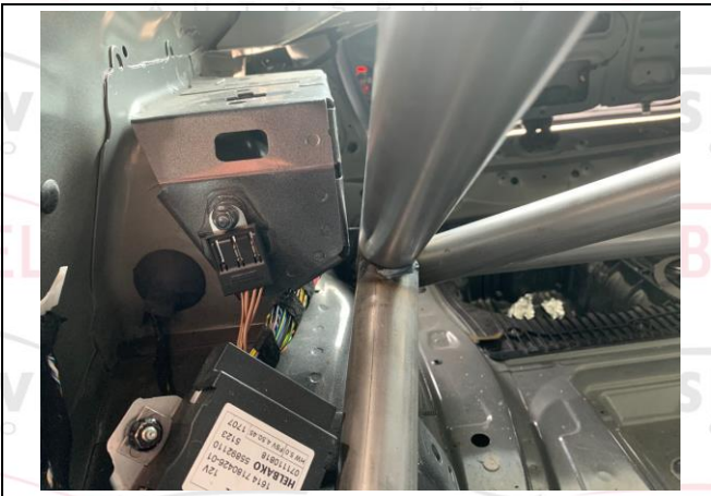
PHOTO 5 REAR BACKSTAY TO BODYSHELL ATTACHMENT
