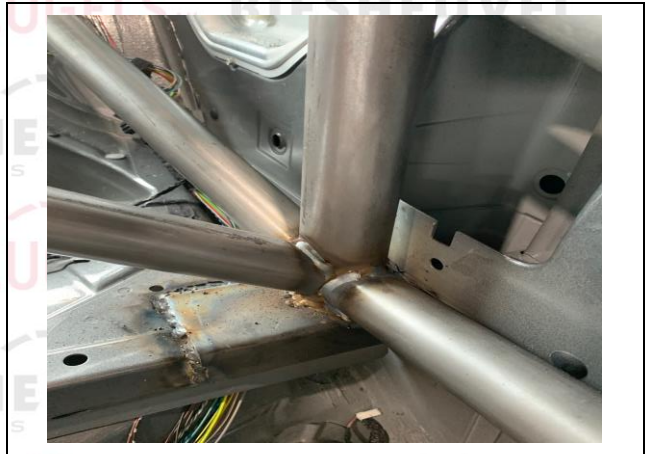
PHOTO 4 MAIN ROLLBAR TO FLOOR ATTACHMENT
